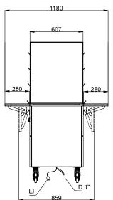
D = Drain El = Electrical inlet (power)
